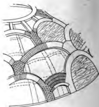
Rib system of dome
